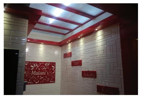
False ceilings are eye-catching and provide insulation against heat because of the gap between the ceiling layers.
